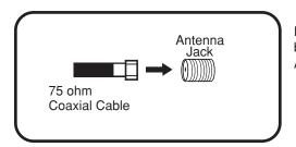
For basic cable service not requiring a Converter/Descrambler box, connect the CATV 75 ohm Coaxial Cable directly to the Antenna Jack on the back of the TV/DVD.
